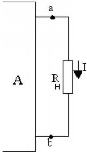
$$I = \frac{U_{xx}}{R_H + R_{вх}} \quad P = I^2 \cdot R_H = \frac{U_{xx}^2 \cdot R_H}{(R_H + R_{вх})^2} \quad (1)$$
